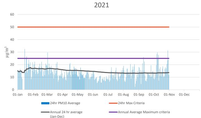
Delta Coals tapered element oscillating microbalance (TEOM) PM10 monitor is located at the Mannering Park Sewage Treatment Plan. No exceedances of the average annual or 24hr criteria have been observed year to date.
